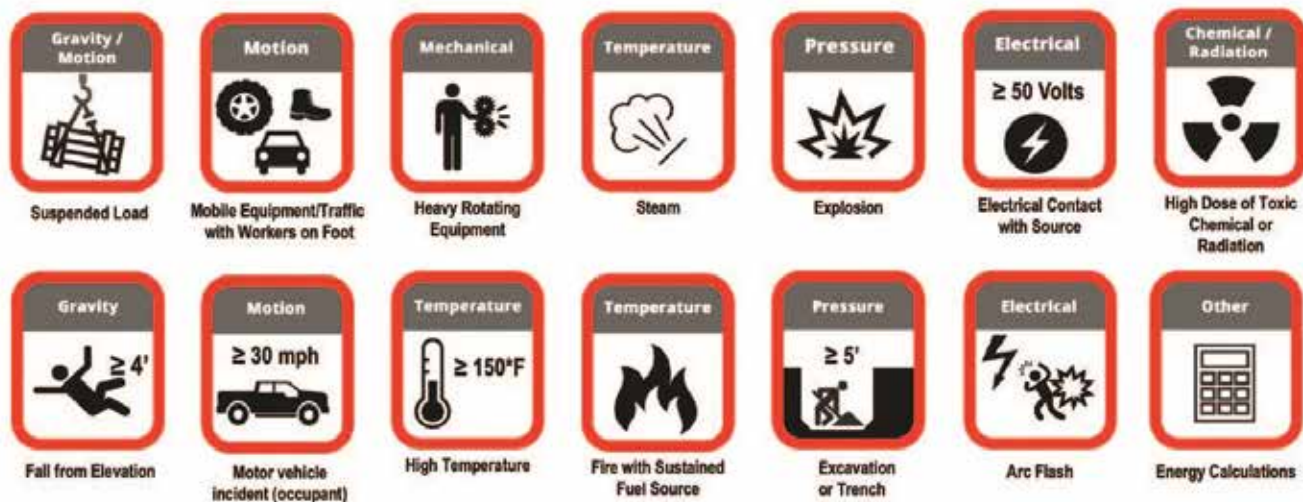
Fig. 1: Examples of High Energy Hazards 5
